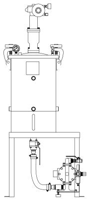
10 Gallon Tank with Diaphragm Pump, Agitator, Vacuum, and Stand
