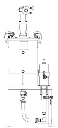
10 Gallon Tank with 5:1 Pump, Agitator, Vacuum, and Stand
