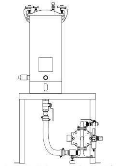
5 Gallon Tank with Diaphragm Pump and Stand
