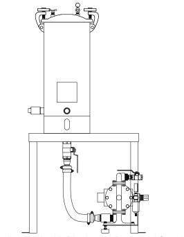
5 Gallon Tank with Diaphragm Pump and Stand
