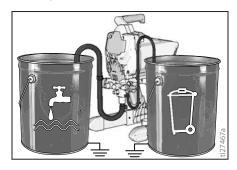
6. Turn Prime/Spray valve down to PRIME position.
