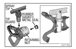
Use spray tip to align gasket and seal in the tip guard.
