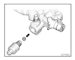
Clean any debris and dried paint from the cavity and replace the ball and spring. Tighten inlet valve to pump using integrated tool on the frame.
