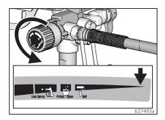
Put drain tube into a waste pail and place Prime/Spray valve in PRIME position (drain) to relieve pressure.
