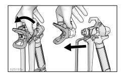
Turn pressure control knob all the way left (counter-clockwise) to lowest setting.
