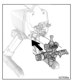
a. Move pump rod up or down until cap is level with the opening in the yoke.
