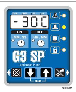
The internal temperature of the unit is out of its recommended operating range.
