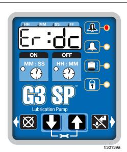
Indicates that a pump has exceeded the 33% duty cycle.
