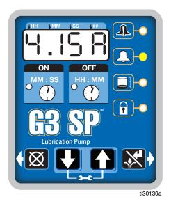
The measured motor current is above the recommended operating maximum value. Continued use at excessive motor currents could reduce life or cause permanent damage.
