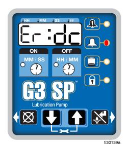
Indicates that a pump has exceeded the 33% duty cycle.
