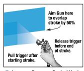
2 Increase Pressure Control Knob if needed until spray is even and without gaps at edges.
