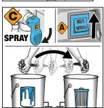
To save paint in hose, disengage Trigger Lock and trigger gun into paint pail, lower Prime/Spray Valve to SPRAY and turn Power Switch ON. When water comes out of gun, keep gun triggered and aim into waste pail. Continue to flush until water runs clear.
