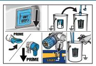
Turn Power Switch OFF. Place Suction and Drain Tubes in waste pail. Move Prime/Spray Valve to PRIME. **Turn Pressure Control Knob** to START position. Trigger gun into a waste pail.
