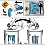
**T**o save paint in hose. **O**disengage Trigger Lock and trigger gun into paint pail, move Prime/Spray Valve to SPRAY and turn Power Switch ON. When water comes out of gun, keep gun triggered and aim into waste pail. Continue to flush until water runs clear.
