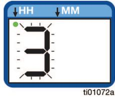
This confirms that the controller is ready for the first digit to be configured for OFF TIME in Hours (HH).
