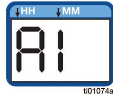
After entering ADVANCED PROGRAMMING, if no activity is detected for 60 seconds, a timeout occurs and the controller resumes RUN MODE.
