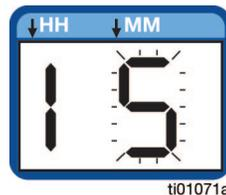
8. Press the UP or Down arrows until the second digit of the PIN Code displays.
