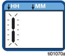
5. Press the UP or Down arrows until the first digit of the PIN Code displays.
