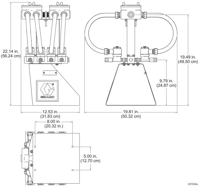
Fig. 6 Multiple-Point Injection Valve Manifold Dimensions
