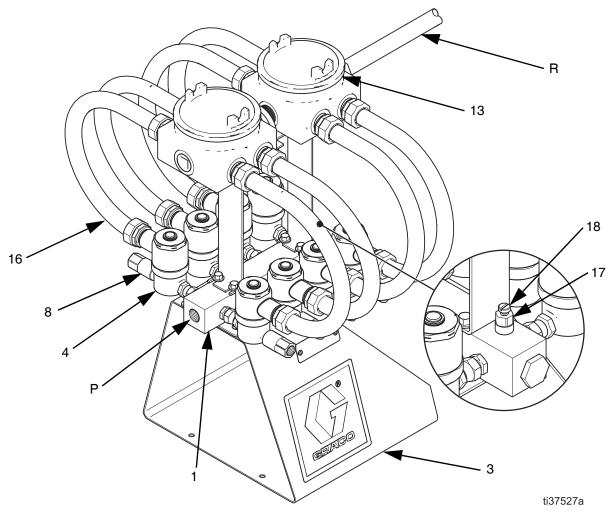
Fig. 1 Multiple-Point Injection Valve Manifold Components
