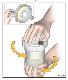
Insert the Funnel into the Cup Lid, twist to lock. Snap the Strainer into the Funnel to strain your paint as you fill your cup.
