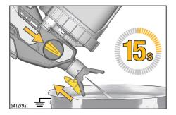
Turn the Spray Tip to the SPRAY position and trigger into a waste pail for 15 seconds.
