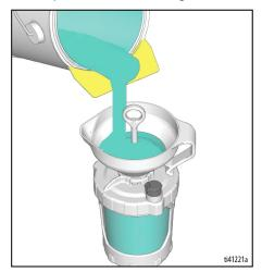
b. With the Funnel and Strainer still attached to the cup, pour excess paint from the Funnel back into the paint can.
