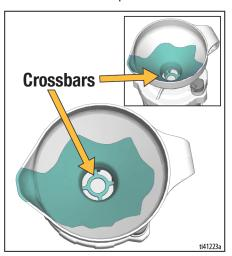
Remove the Funnel and Strainer from the cup and hook on edge of paint can.
