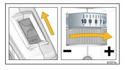
Point sprayer into waste pail, turn Prime Knob forward to SPRAY position. Pull Trigger for 5 seconds to clear clog.
