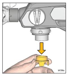
Reinstall the Pump Filter into the pump. Set sprayer on a rag.
