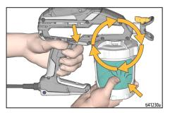
**NOTE:** This will purge all air from the pump and cup. Paint will not spray out, but will recirculate through the pump and back into the cup.
