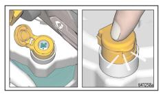
Turn Prime Knob forward to SPRAY position. Verify Spray Tip is forward in the SPRAY position.
